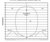
Note: There must be a minimum spacing of 4 mm (0.157 in.) if actuator and sensor face approaches laterally. This will prevent false triggering due to the side lobe areas.
